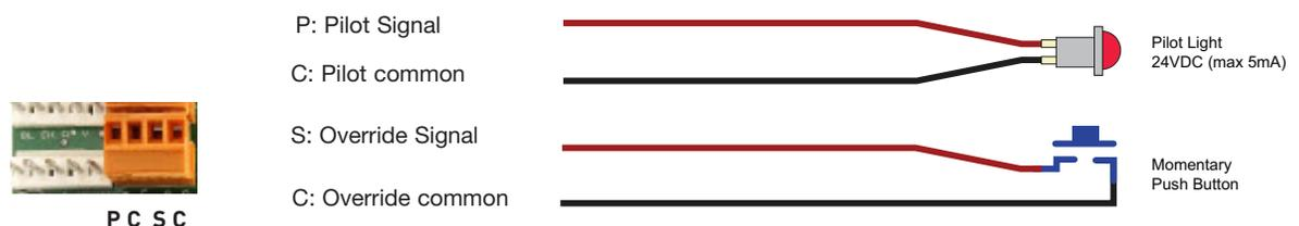
Figure 9: 2-wire momentary switch wiring
